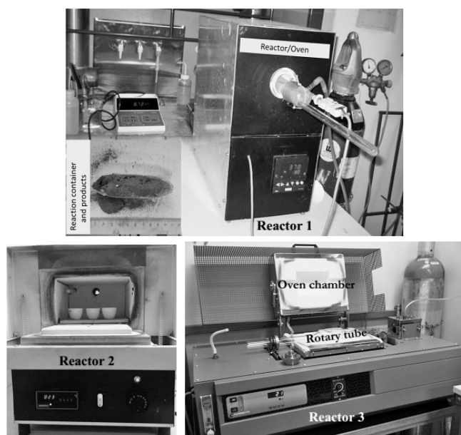
Figure 12 – Reactors used for the solid/solid reaction of magnesium silicates with ammonium salts, at ÅA (taken from Ndguagu (2012)).
