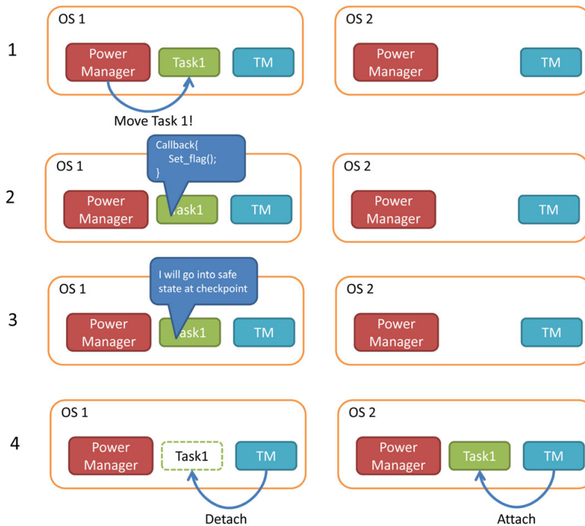
Fig. 3 Request flow in task migration. Left part source core, right part target core
