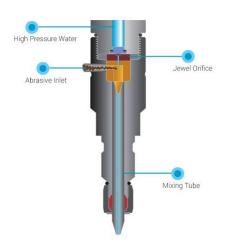
Water jet cutting with maximum pressure water jet technology up to 6000 bar stationarily and 3000 bar mobilely.
