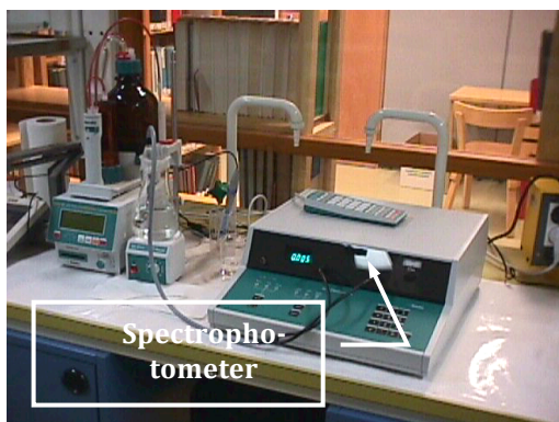
Figure 28. Metrohm Spectrophotometer with a Titrino 751 GPD titrimer (front right), dip in light-electrode (400-700 nm) and Stirrer 728 (back left).
