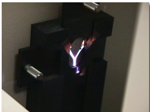
Figure 9. The plasma is reflected to the instrument through a window with a prism behind. The spectre is then passed to a detector inside the instrument.
