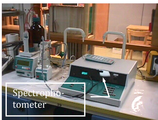
Figure 11. Metrohm Spectrophotometer with a Titrino 751 GPD titrimer (front right), dip in light-electrode (400-700 nm) and Stirrer 728 (back left).
