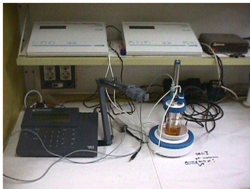
Figure 25. Equipment for conductometric, pH and redox and measurements.
