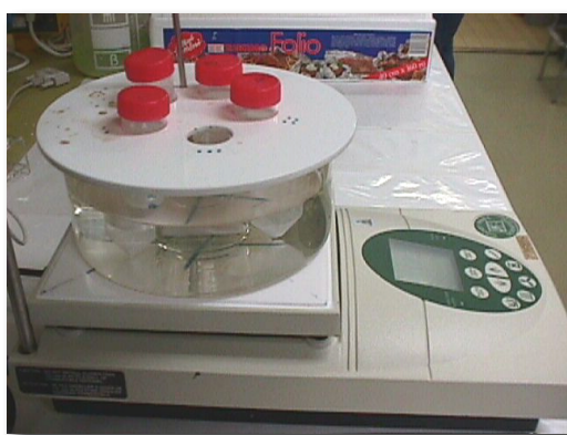
Figure 24. A mini-reactor system/water-bath on a Torrey Pines HS30-2 mixer plate. The plate includes electronically controlled mixer and heater. Each reactor tube (50 ml) contains a small magnet propelled by a larger magnet in the bath, placed in a cut decanter glass in the middle of the vessel.
