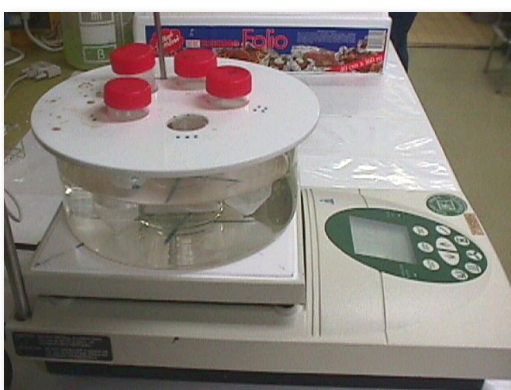
Figure 6. A mini-reactor system/water-bath on a Torrey Pines HS30-2 mixer plate. The plate includes electronically controlled mixer and heater. Each reactor tube (50 ml) contains a small magnet propelled by a larger magnet in the bath, placed in a cut decanter glass in the middle of the vessel.
