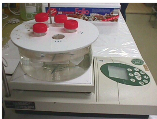
Figure 3. A mini-reactor system/water-bath on a Torrey Pines HS30-2 mixer plate. The plate includes electronically controlled mixer and heater. Each reactor tube (50 ml) contains a small magnet propelled by a larger magnet in the bath, placed in a cut decenter glass in the middle of the vessel.
