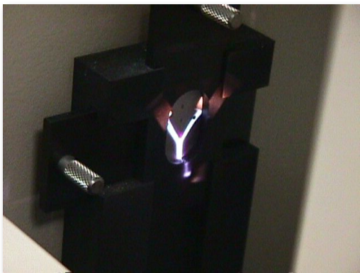
Figure 6. The plasma is reflected to the instrument through a window with a prism behind. The spectre is then passed to a detector inside the instrument.
