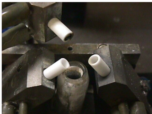
Figure 8. The cathode (up, in the white tube), the anodes (down left and right, in the white tubes) and the sample inlet (down, middle) in the DCP-AES instrument.
