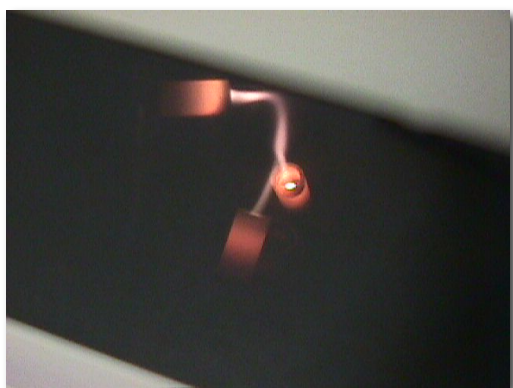
Figure 10. The plasma induced in the ARL Fisons direct current plasma emission spectroscopy instrument model SS-7. The sample is vaporised with an inert gas before entering the plasma zone.
