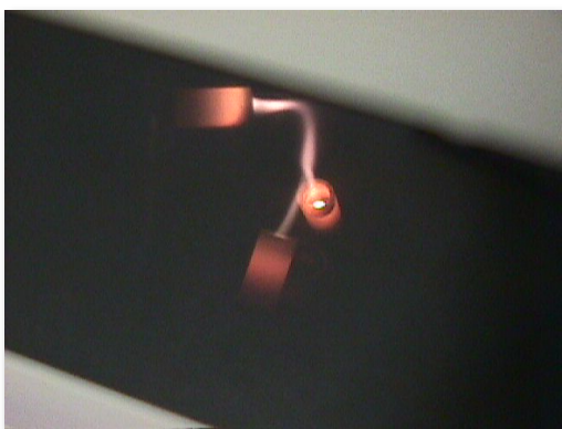
Figure 7. The plasma induced in the ARL Fisons direct current plasma emission spectroscopy instrument model SS-7. The sample is vaporised with an inert gas before entering the plasma zone.
