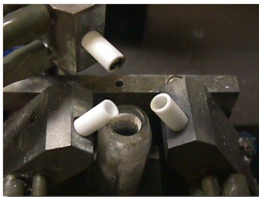
Figure 5. The cathode (up, in the white tube), the anodes (down left and right, in the white tubes) and the sample inlet (down, middle) in the DCP-AES instrument.
