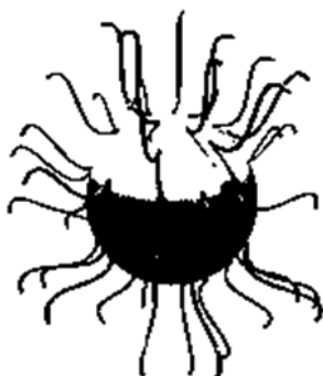
Figure 12. Steric stabilization through adsorbed polymers 69
