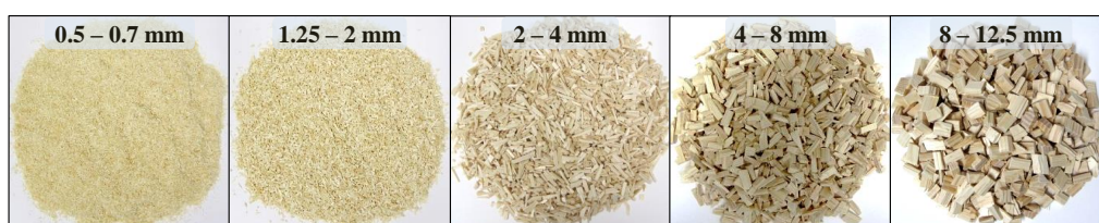
Figure 4.17 Different wood particle size fractions used in the study after milling and sieving.
