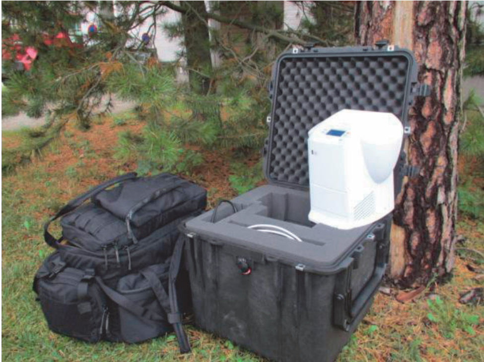
Figure 10. The PikoReal technology equipment was packed into a compact Pelican box with all necessary hardware.
