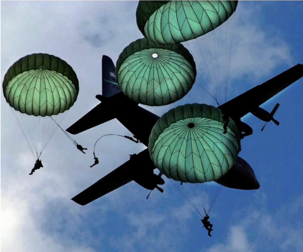
Figure 1. Static line jumping with the T-10 parachute system from a C-130 aircraft. In the middle of the picture a jumper has just exited the aircraft. The arced canopy suspension lines are exposed and the main canopy has been pulled out from its container by the static line (not visible) attached to the aircraft [38]
