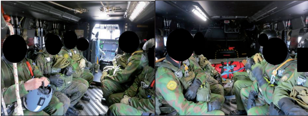
Figure 23. The loading of 13 cabin occupants including: 9 jumpers, 2 jumpmasters, an FTE and the loadmaster (behind the camera). Situation forward of the cabin door is seen on the left aft of the cabin door on the right
