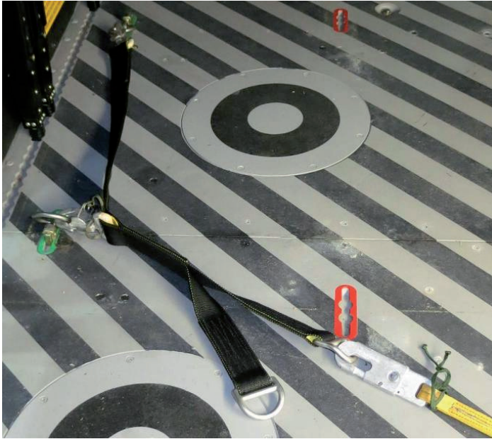
Figure 11. Prototype Anchor for Static line Implementation, version 1 (PASI-1) attached to the front left part of the cabin, onto two “green” attachment points below the row of troop seats. In bottom right, a T-10B static line’s snap hook is shown
