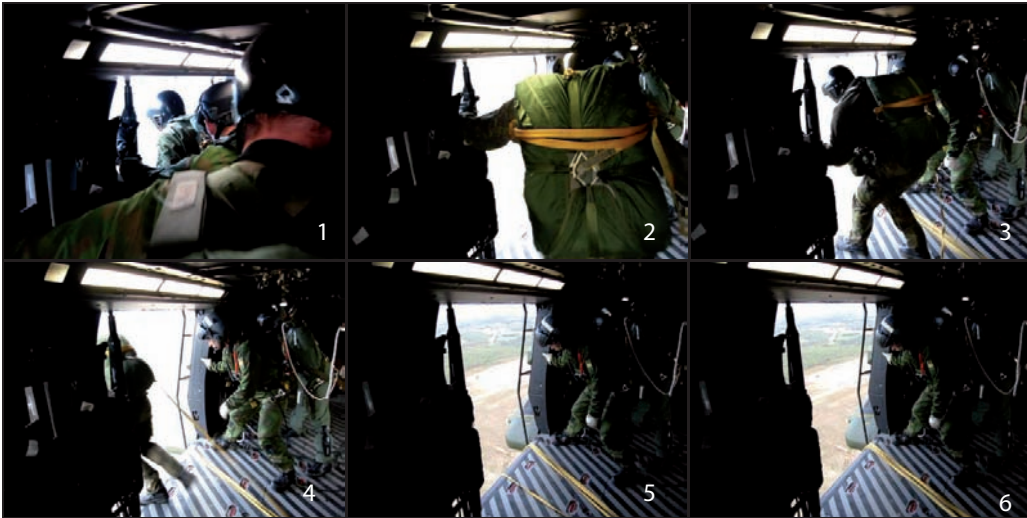
Figure 26. A stick of four jumpers exit at 60 KIAS from a standing position. The top-left picture shows the crowded readiness position. The series from top-middle to bottom-right (steps 2–6) shows the exit of the last jumper of the stick and how the four static lines stabilise below the sponson, contacting also the deflector bar
