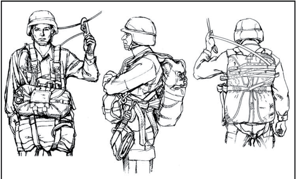
Figure 4. T-10 parachute harness fitted on a paratrooper. The main canopy is on the jumper's back and the reserve canopy on his front. On the left the static line's snap hook is attached to the aircraft via an anchor cable and on the right the static line's folding on the main parachute container is shown [32, p. 2–18]
