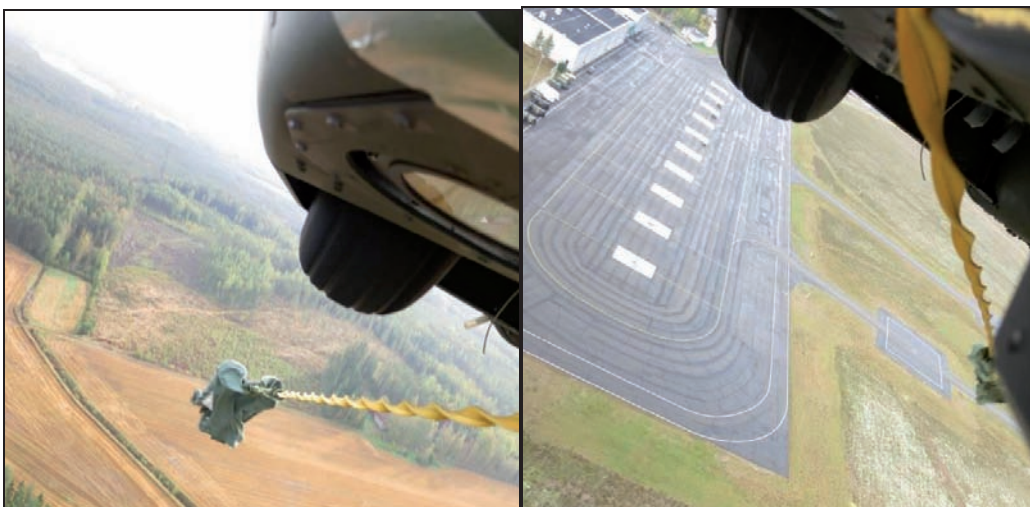
Figure 21. One static line + D-bag below the sponson at 40–50 KIAS with PASI-1. On the left the situation with slip ball on the left (side slipping to the left) and on the right with slip ball on the right (side slipping to the right)
