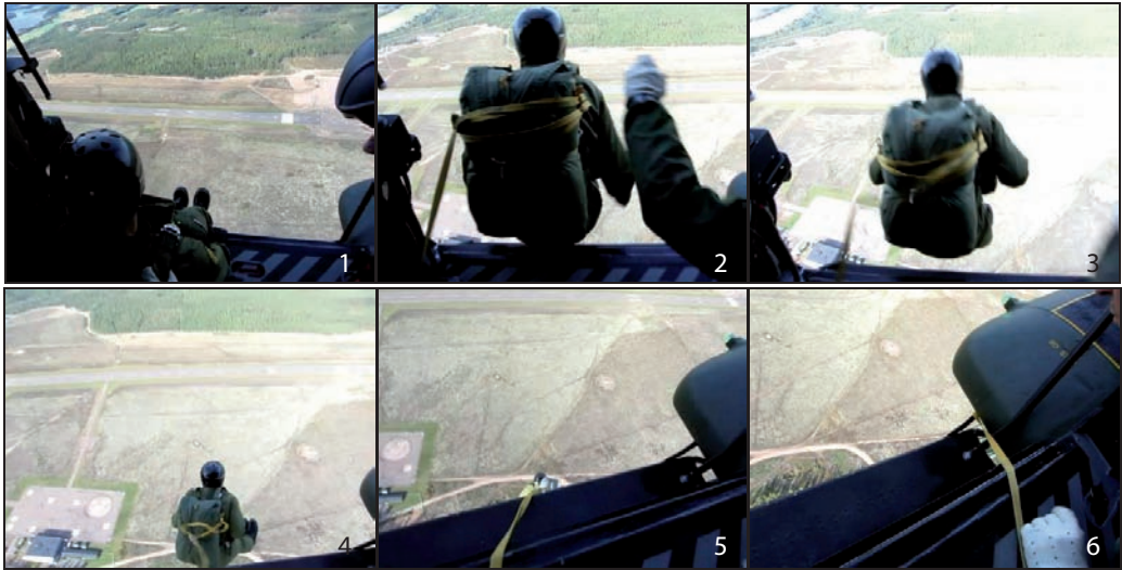
Figure 24. A jumper's exit at 60 KIAS from a seated position. In the readiness position (step 1) the jumper was sitting on the cabin floor facing directly to the side. The feet were hanging outside and hands beside thighs on the door edge. After exit the static line first contacted the middle of the boarding step, then stabilised against the bar between the step and the sponson as seen in step #6 on the bottom right
