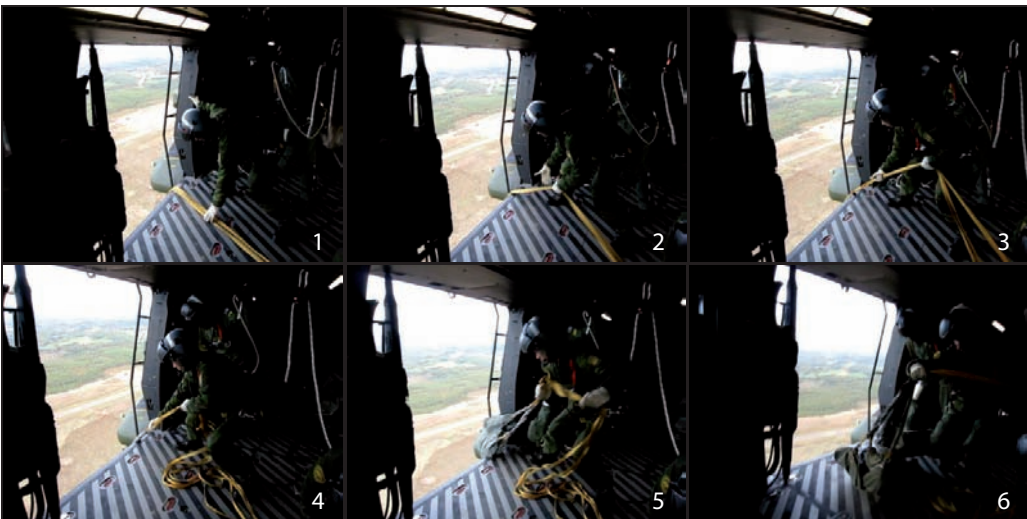
Figure 27. Retraction of four static lines by jumpmaster #1 at 60 KIAS
