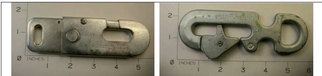
Figure 31. The snap hooks used during the tests. On the left the T-10B snap hook (P/N: MS 70120, proof load 1750 lbs/794 kg/7.8 kN) and on the right the MC1-1C snap hook (P/N: 11-1-6991-1, 100% proof load 1750 lbs/794 kg/7.8 kN, tensile strength 8000 lbs/3600 kg/35.6kN) [25, p. 3-21]. The 11-1-6991-1 snap hook is generally simpler to use as it does not need a safety pin, unlike the earlier MS 70120 snap hook. However, the construction makes the 11-1-6991-1 slightly larger in dimensions.
