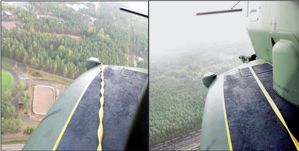
Figure 22. One static line + D-bag above the sponson at 40–50 KIAS with PASI-1. On the left is the situation during side slip to the left (i.e. slip ball on the left). The static line is leaning onto the formation light. On the right is the static line's position during side slip to the right.
