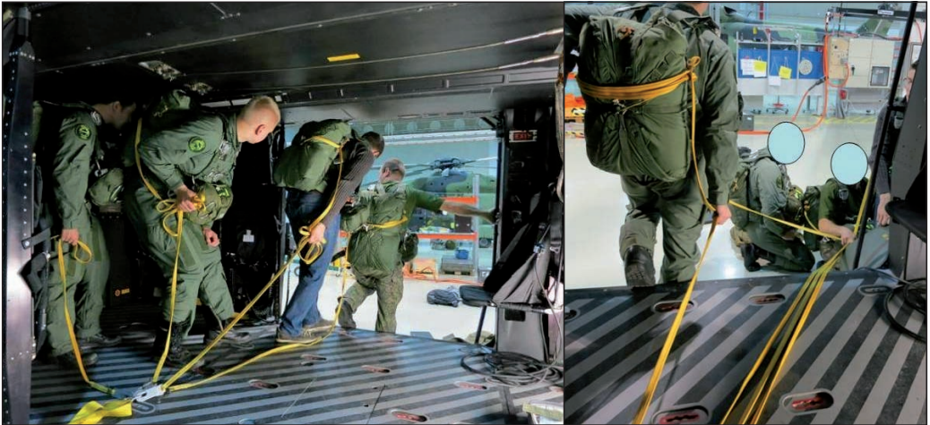
Figure 20. Ground demonstration of a four-man stick exit. Note that the static lines have too much slack in this test situation. On the right is the estimated positioning of the static lines after parachutist separation – there is no interference with the exiting jumpers
