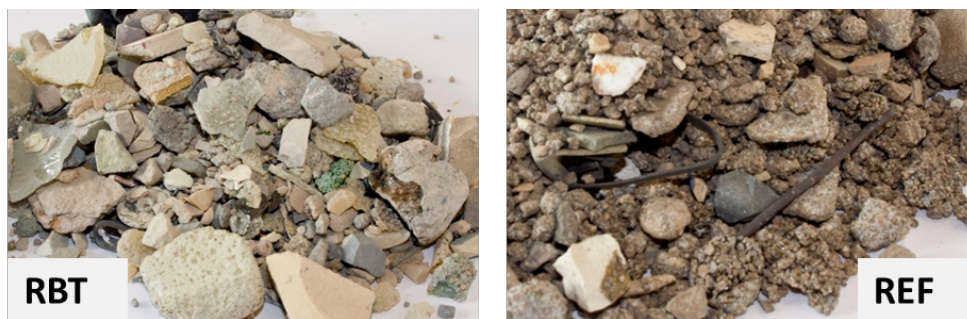
Figure 28. Photos of bed ash for the two different modes of operation of the boiler, Left: Reduced bed temperature case, Right: Reference case with agglomeration (paper VI).
