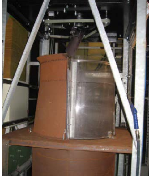
Figure 6. Small-scale model equipment: 1:10 blast furnace charging system (Kjellman 2009).
