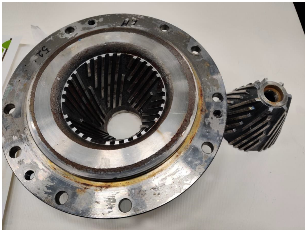
Figure 25b: LM refiner used for refining during the experiment
