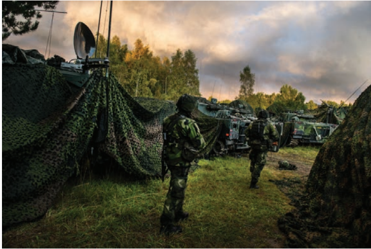
Figure 5-5 Combat vehicles concealed with camouflage nets and soldiers in combat uniforms during a Swedish army exercise in 2015. The camouflage paint on the vehicles, the nets and the uniforms are all examples of spectral design applied to reduce signature. Note that in this picture we can only assess the result in the visible wavelength spectrum since the photographer used a common color camera. Photo: Anna Norén, Swedish Armed Forces.
