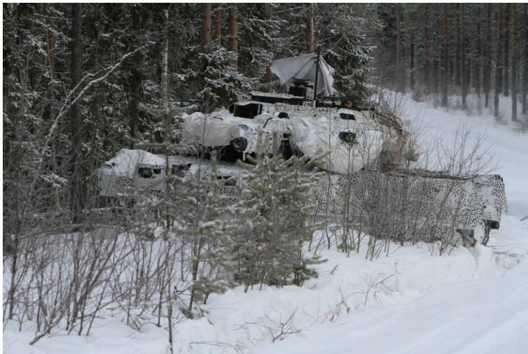
Figure 5-6 Main battle tank during a Mobile Camouflage System (MCS) field trial. Photo: Mats Carlsson, Swedish Armed Forces.
