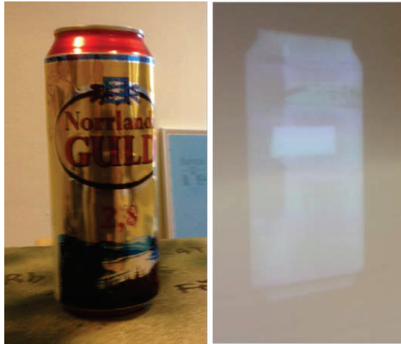
Figure 4-7 Two pictures of the same can filled with hot water. To the left a picture taken with a color camera. To the right a picture taken using the LWIR sensor of the Bill missile system (RBS 56). A small piece of transparent household tape is covering the brand name. Photo: the author.
