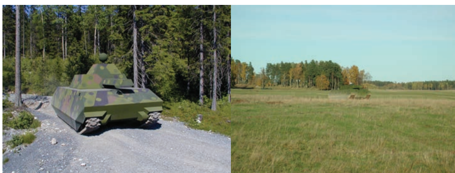
Figure 1. The second low observable technology demonstrator. On the left the characteristic low radar signature shape of the vehicle is prominent. The picture on the right demonstrates the visual signature at a more tactically relevant distance. Photos courtesy of BAE Hägglunds AB and of Saab Barracuda AB respectively.
