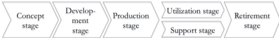
Figure 4-1 The generic life cycle of a system according to ISO/IEC/IEEE 15288:2015
