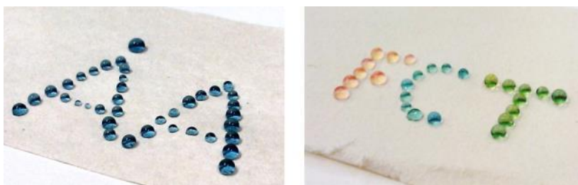
Figure 3.2 Examples of functionalised, i.e. hydrophobic, laboratory hand sheets.
