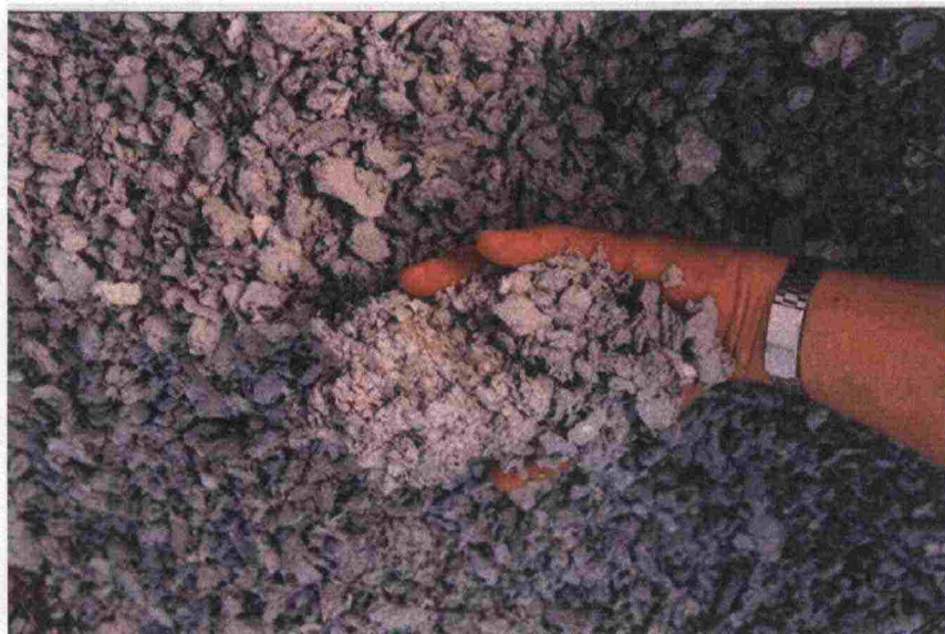
Figure 4-8: Fibre-sludge or "fibre-clay" consists of organic fibres, kaolin and water.
