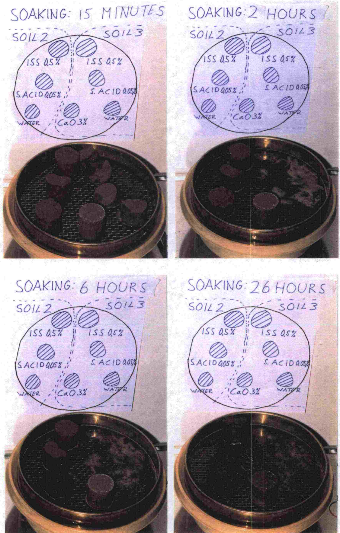
Figure 21. Behaviour of the specimens of the Zambian clays in the soaking test when they were air-dried after 75 days of moist curing. The soils are from the district road D154 near Lusaka.
