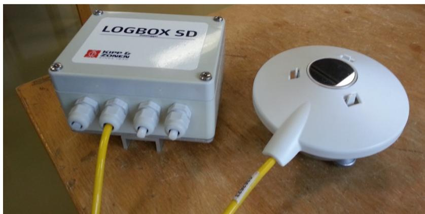
Figure 6. Picture of used pyrgeometer
