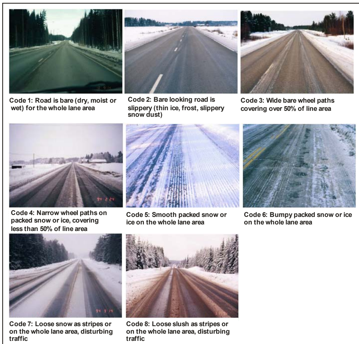
Figure 4. Road weather classification used in this study. Based on the "centralized winter maintenance control" classification.
