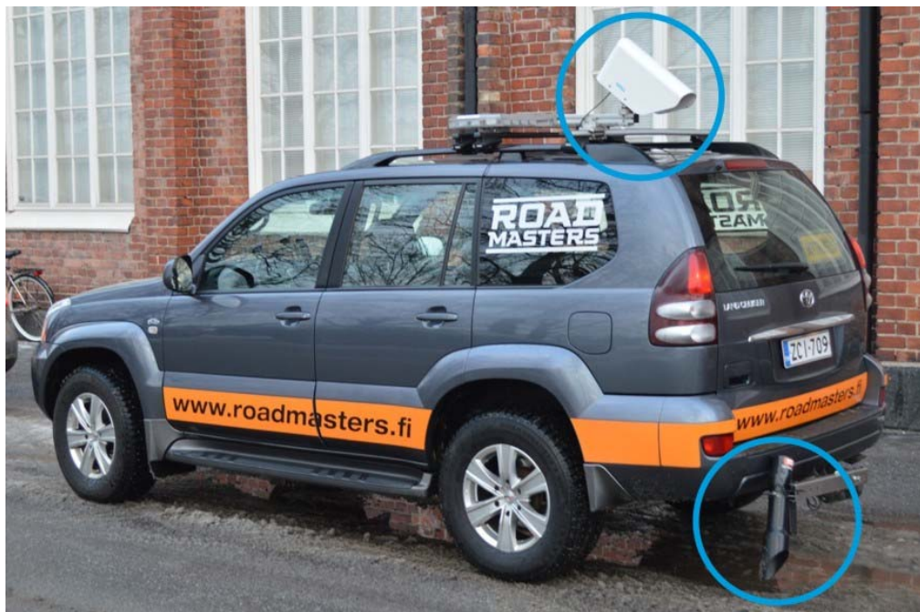
Figure 1. Optical friction meter DSP310 (in the blue circle above) analyses the road surface farther and should be detached on the roof stand. Optical friction meter RCM411 analyses the surface nearer and is here detached on the towing hook. Both meters are focused on the left wheel path.
